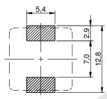
no vias and sensitive traces underneath the component Scale - 2:1
