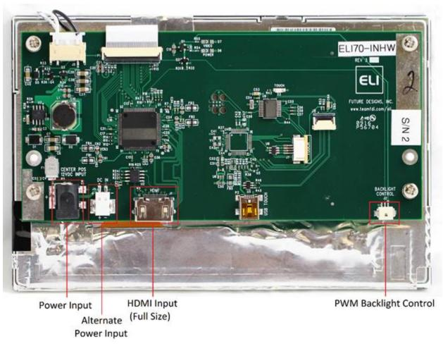
Power may be supplied either via the 2-pin terminal block J4 or via the 2.1mm power jack P2 (center positive)
